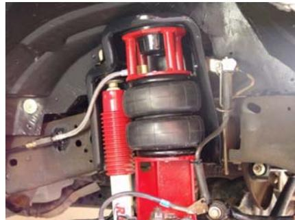
7. Install the air bag assembly just as the coil spring came out. Use the original lower mounting bolt and supplied spacer to attach the lower mount to the axle housing.
