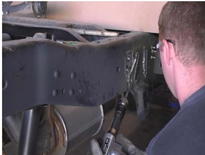
11. Grind the frame smooth and install the spring hanger in the existing rivet holes. Drill the frame for the 2 holes on the bottom of the frame and tighten the mounting bolts
