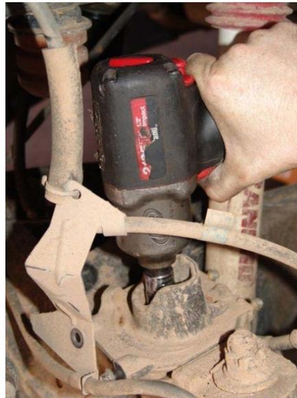
5. Remove the bolt that attaches the lower coil spring seat to the axle housing. Set the bolt aside as it will be used again during reassembly
