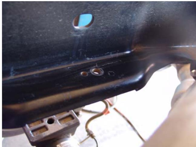
17. Align the large elongated hole on the upper bag mount with the one on the frame. Mark and drill mounting holes in the frame and install the inner and outer halves of the upper bag mount
