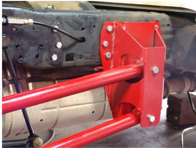
7. For 08 and newer trucks, hanger removal is more difficult, since the hangers are riveted and welded on. It is important that the hanger is removed without damaging or affecting the structural integrity of the frame. Make sure a qualified person performs the next few steps
