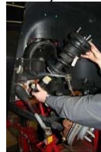
OEM upper strut studs and torque to manufacturer's specifications.
