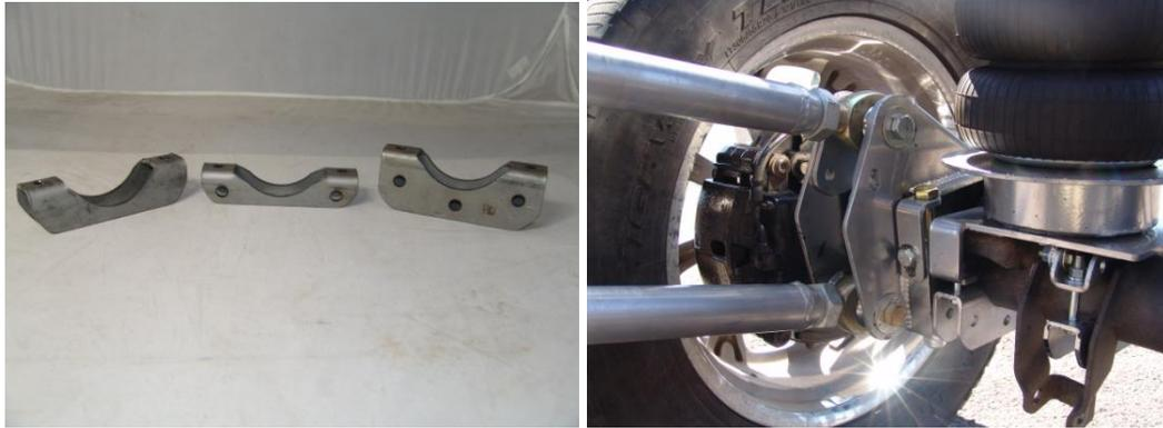
16. Install air fitting on airbag and mount the rear air bags. Be sure to place the 9 ½” diameter flat bag plate between the bag and bag mounts. This keeps the bag from rolling over itself at low pressures and contacting any sharp objects.
