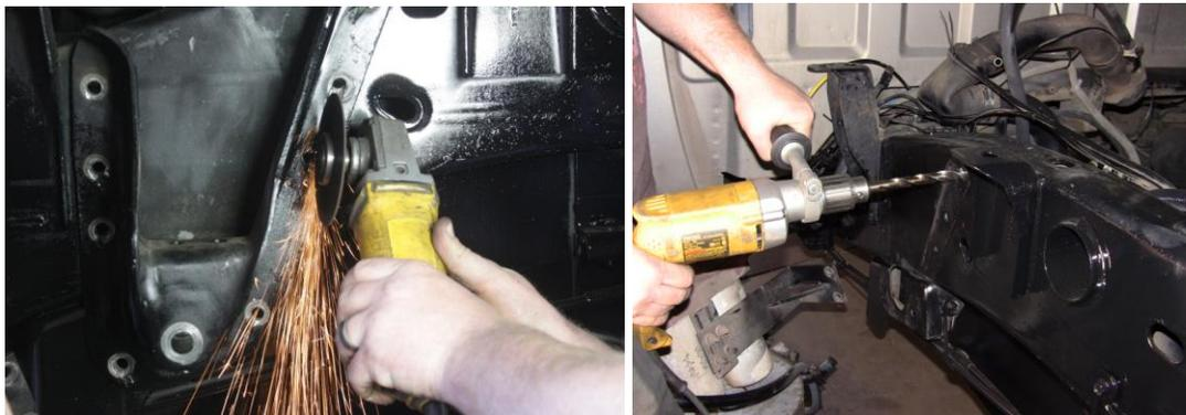
7. Install the new 4 link mounts. The 4 link mounts install into the factory leaf spring hanger's mounting holes
