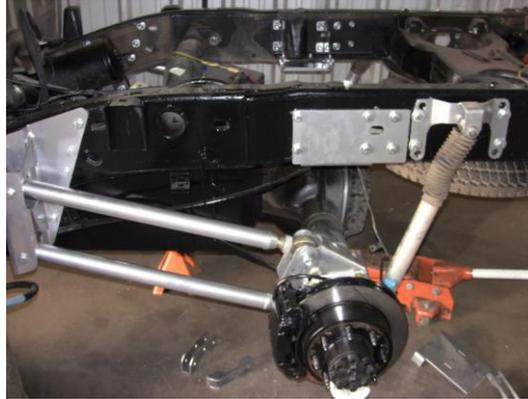
18. Be sure to tighten all hardware after installation for the hangers, links, axle mounts, bag brackets, shock brackets, pan hard bar and differential bracket. Check again after 50 miles of driving
