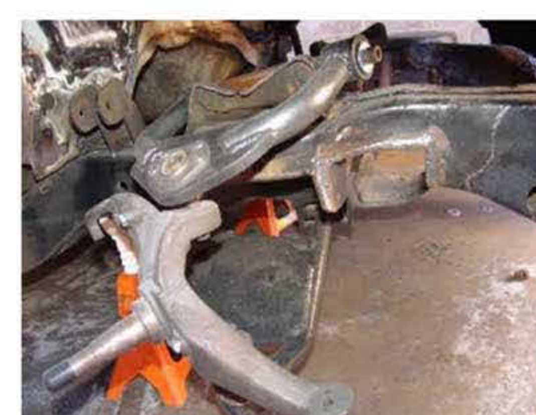
Passenger side with control arms installed and spindle turned to the right. Passenger side with control arms installed and spindle turned to the left. If you are installing Optional Spring Pocket Eliminators,
