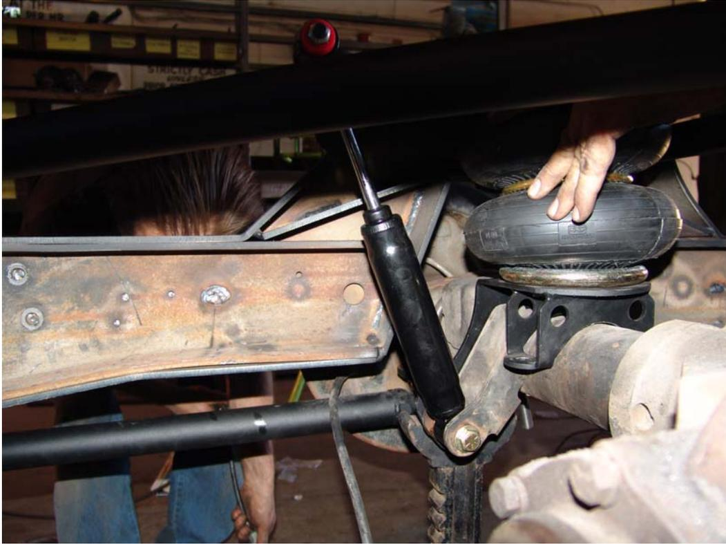
Passenger side lower over axle bracket & shock installed
