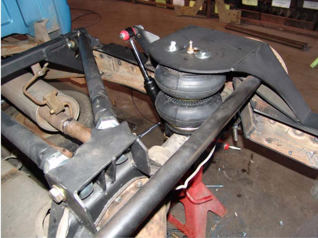
Passenger side showing diff bracket, rear cross member & bag installed
